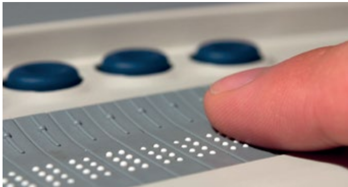
The Braille display is an assistive device for using computers by blind people.
